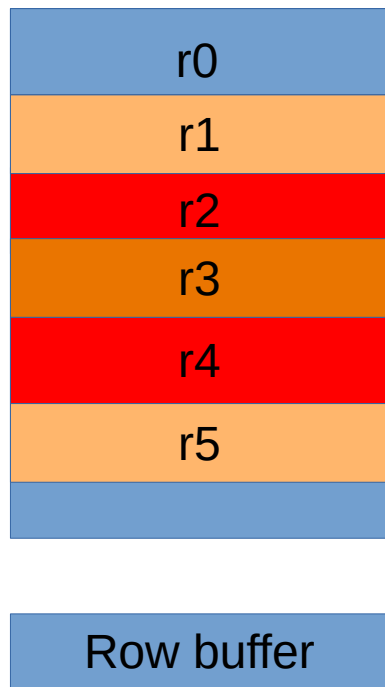
Double sided hammering
